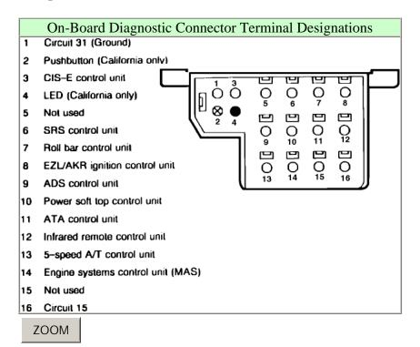
The on-board diagnostic connector provides information concerning fault conditions within the CIS-E(5), SRS, EZL/AKR, MAS, Electronic A/T
