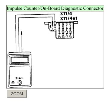
When the start-button on the impulse counter is depressed for 2 to 4 seconds (ignition ON), the impulse counter will begin a impulse readout. The cause of the malfunction(s) will be indicated by the number in the impulse counter window. Fault codes will be displayed in ascending order. If several fault codes are stored, the next fault code will be displayed by pressing the start button again. If no additional fault codes are stored, the first number will reappear.
